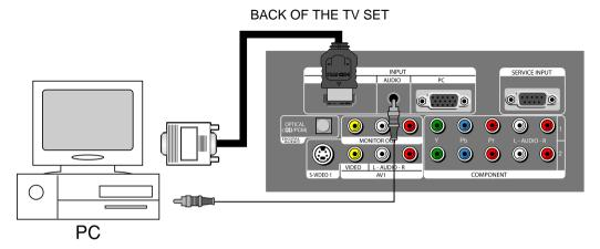
**Note:** If the graphic card of the PC only supports a DVI signal, you must connect the Audio cable like above the picture.
